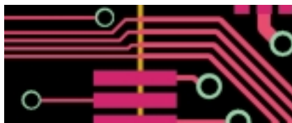
Figure 4. Rules by Area. Another approach to routing in congested device pad areas is to define different, smaller rules within a limited region.
